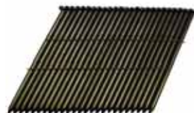
Clipped Head Strip, 28° Wire Collated 2" x .113 to 3/2" x .131
